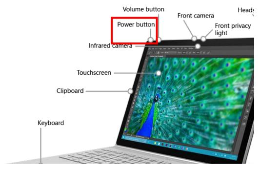
1. Power on the device. The button is located on the outside edge of the screen, on the upper left.
